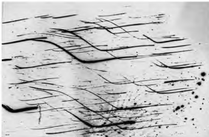
FIG. 28. (2:R) Curve Swarm Group of correlated tracks exhibiting smooth curvature. Note that tracks curve in both directions. Note also that these are white tracks on a black background. That is, these tracks are formed by a tearing down or bleaching of the latent image. A charged particle in an applied magnetic field (and no other applied fields) is expected to curve in only one direction according to the sign of its charge.
